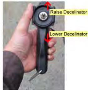
Lower the Decelinator by pushing the toggle switch down.
