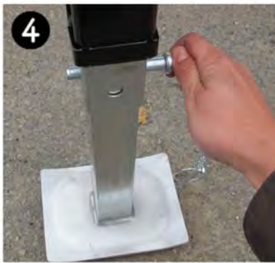
4 Remove drop leg pin from drop leg.
