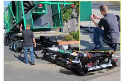
Fold the steel ramps back to the towing position.
