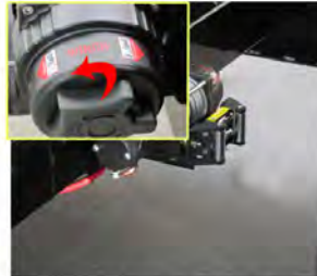
Turn the trailer's winch counter-clockwise to the "Engage" position. Hold the "IN" button on the controller to slowly bring the Decelinator onto the trailer's track.
