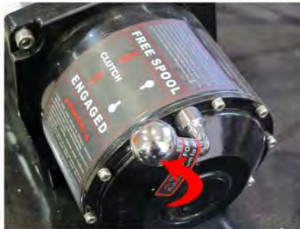
Activate the "Engaged" option on the Winch by pulling the lever towards you or where it is indicated on the winch.
