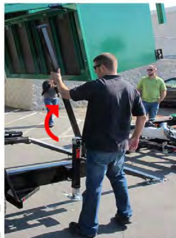
Raise the steel ram stop, bolted to the trailer, underneath the Zippin Zone platform. Lower the platform onto the ram stop.
