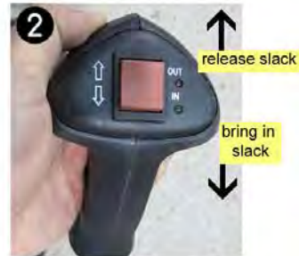
2 Push the button down, "in" position, to bring in the slack.
