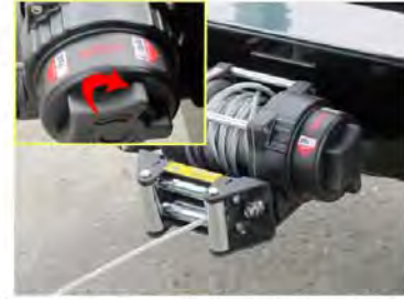
Free the spool on trailer's winch. Press the "out" button to release the cable slowly to the ground.
