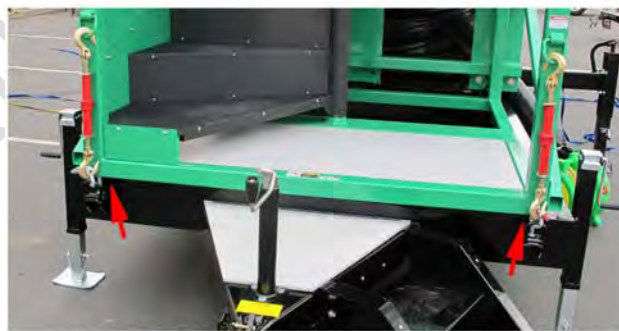
The Zippin Zone Platform in the operational position resting on the platform stops.
