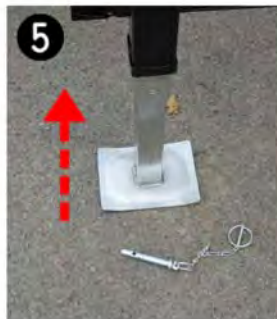
5 Push drop leg up into jack and securely fasten the leg pin back into place.
