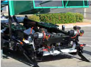
Slowly release the slack from the winch to lower the Decelinator to the ground.
