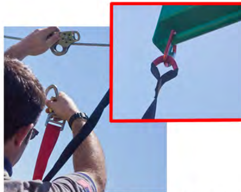
Wear a Speed Harness and use the lanyard (black) to connect to the center beam, between the zip cords. Always be securely attached with a safety lanyard during operation.
