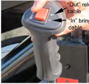
Button can either bring in "IN" the cable slack or "OUT" release cable from winch.
