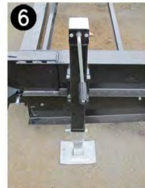
6 Ensure that the jack rests firmly on the ground, not raising the tires off the ground.
