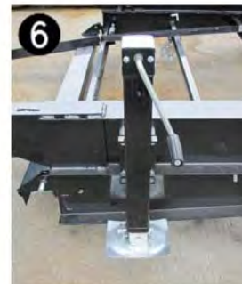
6 Continue to raise the jack, counter-clockwise, until you no longer can bring up the drop leg.
