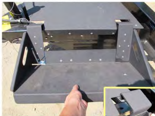
Unhook the staircase into the notches located on the side of the tongue of the trailer.
