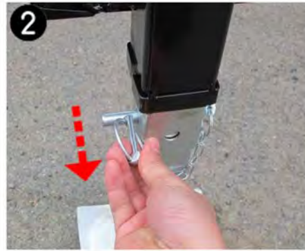
2 Pull safety lock clip from drop leg pin.
