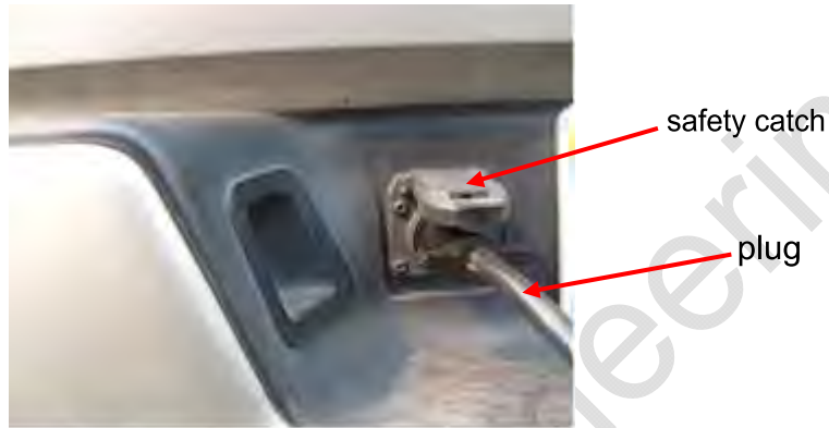
Electrical Towing Plug properly inserted into tow vehicle socket with socket cover safety catch down over trailer plug
