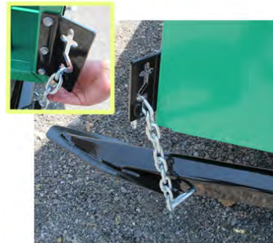
Attach the safety chains to the brackets to hold the ramps in place. Bring in all of the chain slack to hold the ramps as far up as possible.
