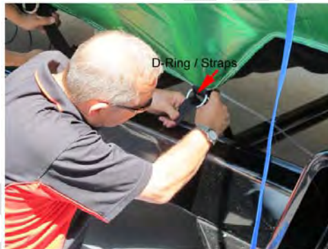
4 D-Rings are located on the base of the inflatable to securely fasten the slide to the trailer's load hooks.
