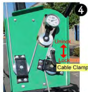
4 Lock the cable clamp next to the gauge, to prevent the cable from releasing slack.
