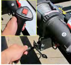
Plug in the winch controller.
