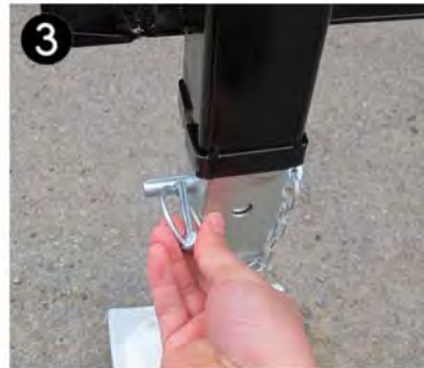
3 Pull safety lock clip from drop leg pin.
