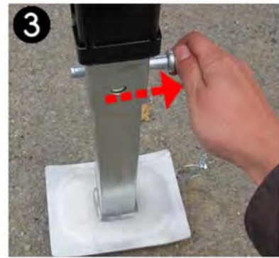
3 Allow drop leg to rest on ground and replace pin back into drop leg.
