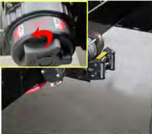
Turn the trailer's winch counter-clockwise to the "Engage" position. Hold the "IN" button on the controller to slowly bring the cable slack. Remove the controller and safely store away.
