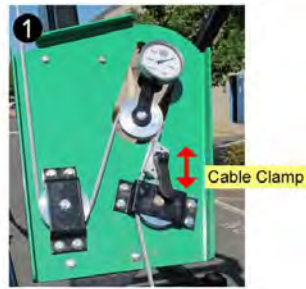
1 Unlock the cable clamp next to the gauge, releasing slack.
