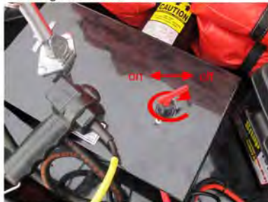
Plug in the Decelinator's lift controller (yellow cord) and make sure the emergency switch is not on.
