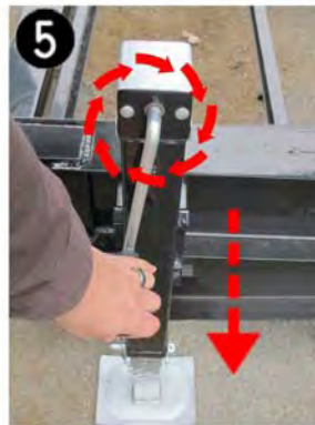
5 Turn jack handle clockwise to lower the jack leg to the ground.
