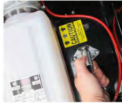
Remove the lift controller. Do not pull from the cord. This can damage the lift controller.
