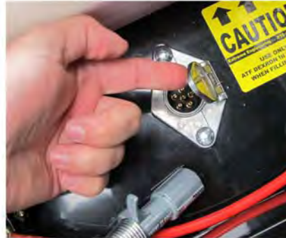
Raise the protective cover off the socket to attach the lift controller.
