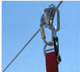
Take the black lanyard from the handrail and then connect it to the backup zip line pulley attachment. Make sure the zip cord is through the carabiner.
