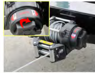
Free the spool on trailer's winch. Press the "out" button to release the cable slowly to the ground.
