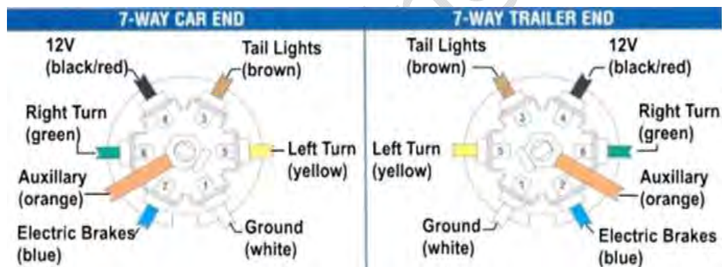
RV 7-Wire Wiring Diagram
