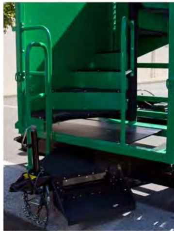
Final view with staircase installed and Zippin Zone platform raised.
