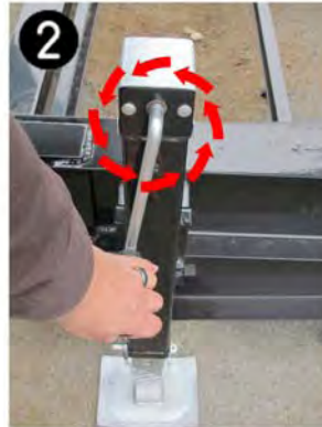
2 Turn jack handle counter-clockwise to raise the jack leg off the ground.
