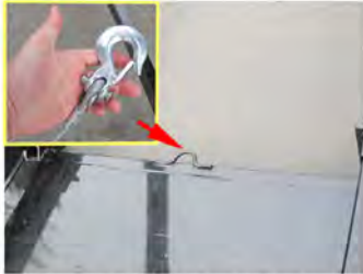
Connect the winch's hook to the front load hook on the Decelinator.
