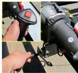
Plug in the winch controller.
