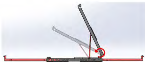
Lower the Decelinator until the lift rams can no longer lower the the Decelinator to the platform. DO NOT remove zip cords before lowering!
