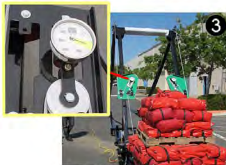
3 Set the tension between 1,000 to 1,300 lbs on the gauges for the correct operating zip cord tension.
