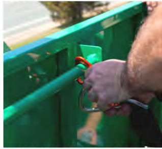
Connect the participant to the hand rail with the black lanyard.
