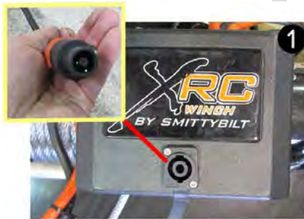
1 Locate the socket on the winches and align the winch controller's plug with the socket. Plug the controller into the socket.
