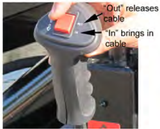
Button can either bring in "IN" the cable slack or "OUT" release cable from winch.
