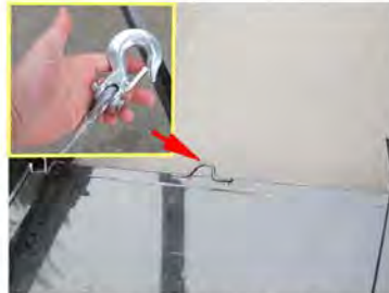
Once the Decelinator is firmly resting on the ground, remove the winch's hook from the load hook on the Decelinator.
