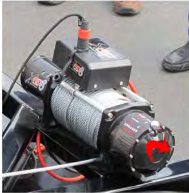
Ensure that the winch is in the "Free Spool" position when raising the Zippin Zone Platform.
