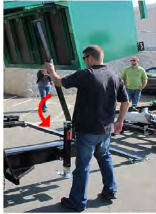
Slightly raise the tower and lower the steel ram stop back onto the trailer. Lower the tower back onto the trailer.
