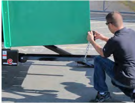
Disconnect the loading ramp safety chains from the tower's brackets on both sides.
