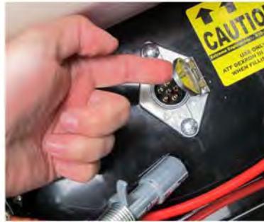
Raise the protective cover off the socket to attach the lift controller.
