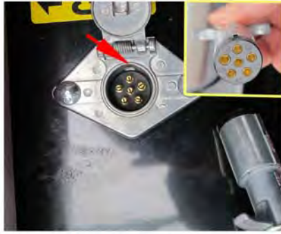
Raise the protective cover on the lift pump and grab the steel end of the lift controller .
