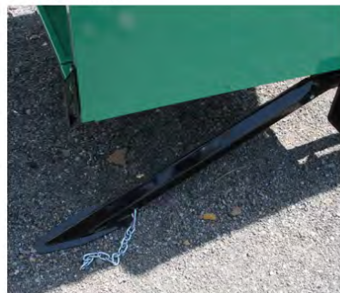
Raise the ramps to the towing position.
