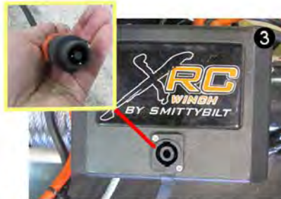
3 Locate the socket on the winches and align the winch controller's plug with the socket. Plug the controller into the socket.
