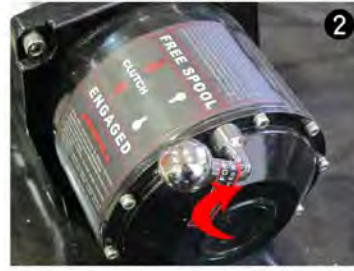
2 Activate the "Free Spool" option on the Winch by pulling the lever towards you or where it is indicated on the winch.
