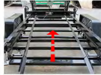
Carefully bring the Decelinator onto the Zippin Zone's trailer by ensuring the Decelinator loads onto the track. Stop until you can no longer bring in the winch's slack and the Decelinator onto the track. Remove controller and safely store away.
