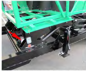
Locate the lift pump between the two lift rams, towards the tongue of the trailer.
