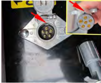
Make sure to align the notch on the plug with the socket to successfully insert the controller.
