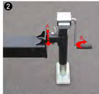
2 Ensure that the stabilizing jacks are properly attached to the outriggers and the legs are resting firmly on the ground. Pin the jack into place and turn the jack handle clockwise to lower the drop leg.
