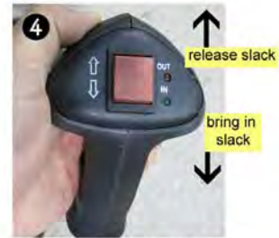
4 Push the button down, "in" position, to bring in the slack and roll cable along the spool until you no longer can bring in the cable on the winch. Repeat on 2nd zip cord.
